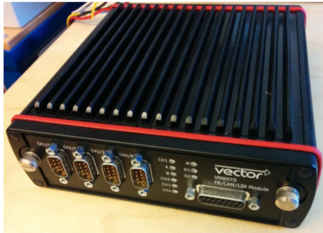
Figure 3-1: VN8970 real-time system from Vector Informatik GmbH for simulating the CAN-network in which the ECU will later be used. Figure by A. Karlsson [23].
